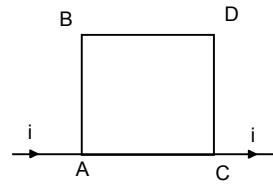
20. For AB  $B$  is along  $\odot$   $B = \frac{\mu_0 i}{4\pi r} (\sin 60^\circ + \sin 60^\circ)$
