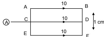
$$30. \frac{\mu_0 i_1 i_2}{2\pi d} = mg \text{ (For a portion of wire of length 1m)}$$
