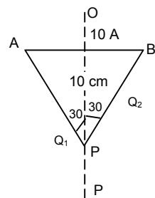
$$16. B_1 = \frac{\mu_0 i}{2\pi d}, \quad B_2 = \frac{\mu_0 i}{4\pi d} (2 \times \sin\theta) = \frac{\mu_0 i}{4\pi d} \frac{2 \times \ell}{2\sqrt{d^2 + \frac{\ell^2}{4}}} = \frac{\mu_0 i \ell}{4\pi d \sqrt{d^2 + \frac{\ell^2}{4}}}$$
